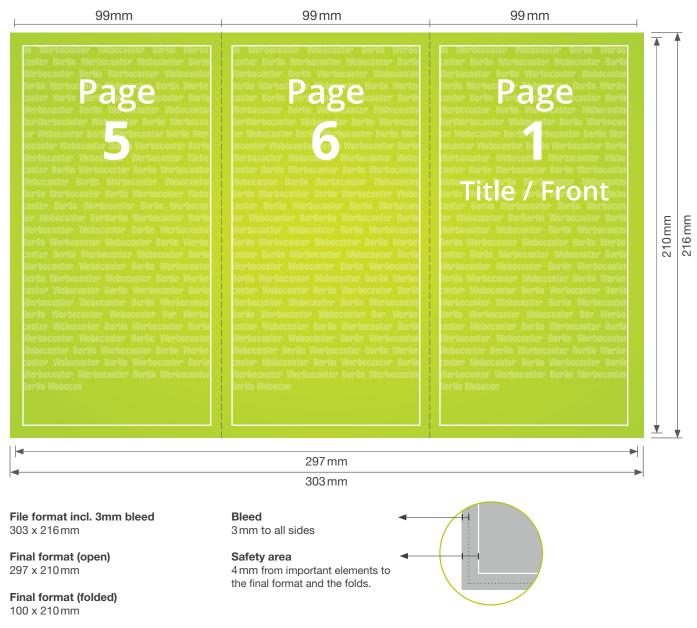
We recommend a safety space of 4 mm for text, logos or other important elements. For the cut we could not garantee precisely sizes by millimeter.
