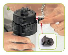
Fix the suspension hook at the telescopic bars. If you want to use the graphics in a angle of 90°, it is recommended to attach the hanger at the base of the rod before you fix the foot base.
